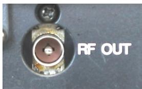
*Here is the antenna output of a video recorder.*
