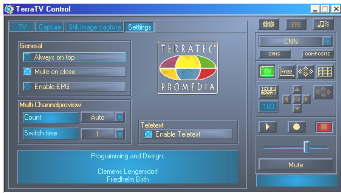
**General.** If you select the option “Always on top”, the remote control does not disappear behind another window or behind applications, but instead it stays on. This setting only applies to the remote control. You can separately select such an option for the Teletext or Video window.
