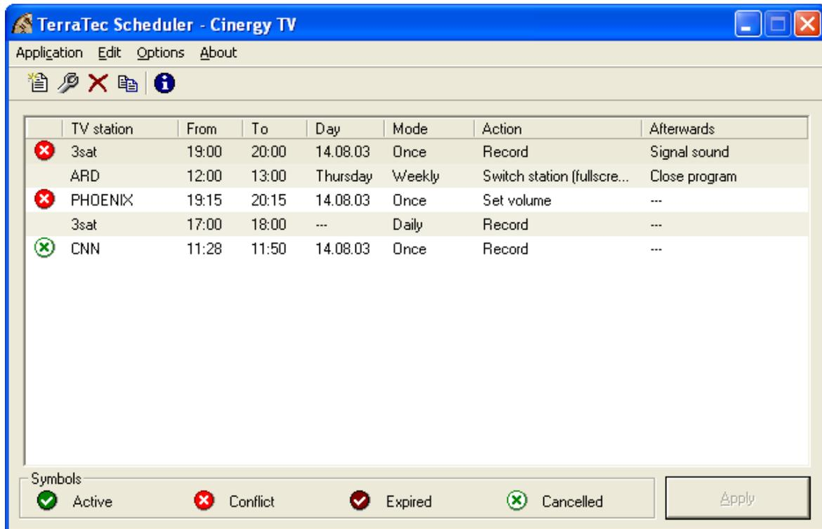
As the Cinergy cannot receive more than one station at a time, the entries in the first and third row provoke a conflict as the radio is set to record one program from 19:00 to 20:00 and another from 19:15 to 20:15. The Cinergy would have to switch over at that moment, canceling the first recording.
