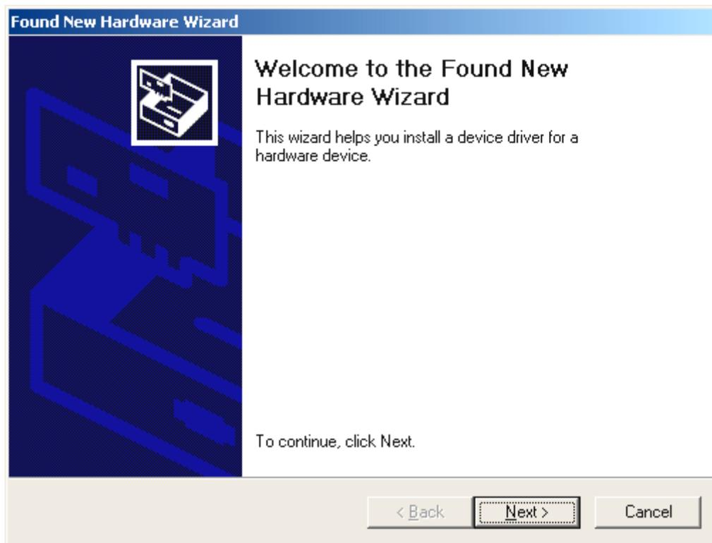
*Windows 2000 automatically detects the presence of a new hardware component in the system and tells you so in a subsequent window, which you confirm by clicking “Next >”.*
