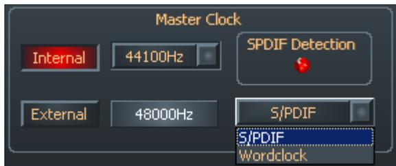
DAT recorder) or it can set a sampler rate itself and provide this signal to other devices. When choosing “Internal”, you can choose from all commonly used sample rates from 32 to 96 kHz—the actual bit rate is not important at this point. The external
