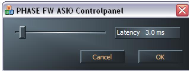
Panel. The ASIO latency (in ms) is directly related to the processing speed of the ASIO driver; if this value is too low, it can adversely affect the performance of your system as a whole. With a fast system, you should
