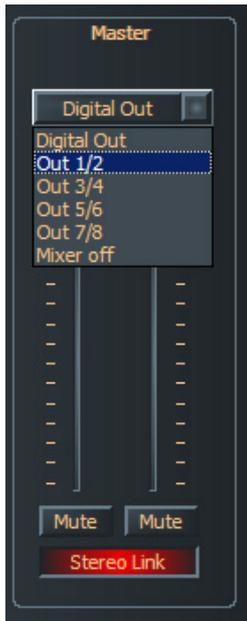
Level, panorama and mute controls are also available for the mixer's master output. The PHASE 88 Rack FW outputs available for the mixer output can be selected above the fader. The waveplay stereo channel assigned to the output by default will be switched off.
