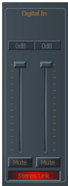
“Digital In” is grayed out until a valid digital signal is applied to the digital input and the Master Clock is set to “External”.
