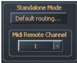
With the MIDI Remote Mode, the digital hardware mixer and the signal router can be controlled in real time with a MIDI fader box or any other MIDI controller that can send MIDI control changes and is connected to MIDI In port 2. The MIDI settings used by the device are defined by the Control Panel via 1394. The MIDI channel that is monitored by the device is specified by a combo box in the control panel.
