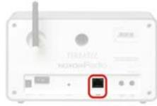
Use a standard network cable to connect the device to a router, switch or hub—to connect it to your PC directly, use a crossover cable.
