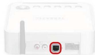
The output uses the **S/PDIF** (Sony / Philips Digital Interface) protocol. This is a standard protocol for digital transmission of audio signals, and it is supported by just about any device with a digital interface.
