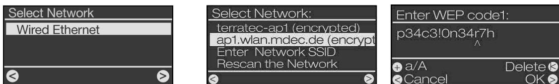
**A)** If you have used a cable to connect the NOXON (Wired Ethernet), the installation is very simple, since you do not require a network key. Confirm the selection again with ►.
