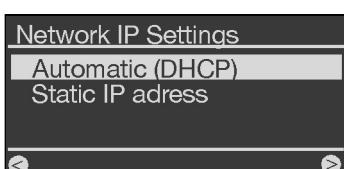
**3)** Acquiring the IP address (kind of like a "home address" for your network): If you are unsure, simply select 'Automatic (DHCP)'. This is the correct setting for most users, as in this case the router assigns the IP address itself. If you want to assign a static IP address to your NOXON, select the corresponding entry. For more information, refer to your manual.
