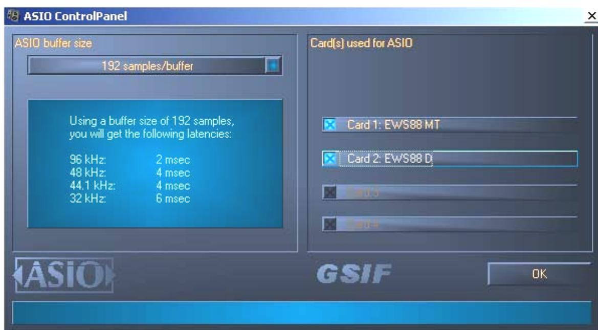
The ASIO driver is listed in compatible programs under “ASIO for EWS88 MT/D”. The inputs and outputs (generally “busses”) available in the programs are called “EWS88 MT (n) Out”, wherein “n” is used to distinguish multiple EWS MIC systems (1 to 4). In many cases only the left channel of the output pair (1/2, 3/4, 5/6, 7/8 and S/PDIF Left/Right) is stated, it applies for both channels however.
