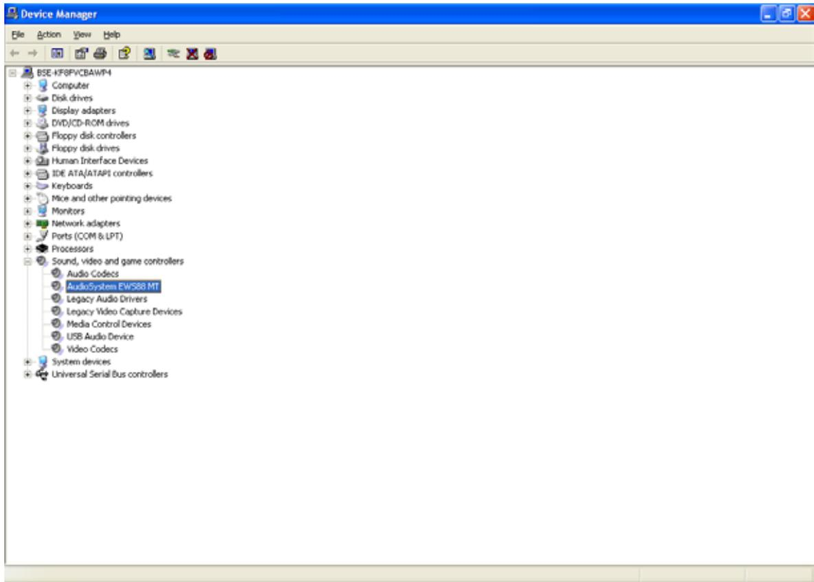
*If everything is correctly set up, the window should look like this. The figure shows the expanded view of the “Sound, video and game controllers” branch. To obtain this view, simply click the “+” symbol on the left side.*
