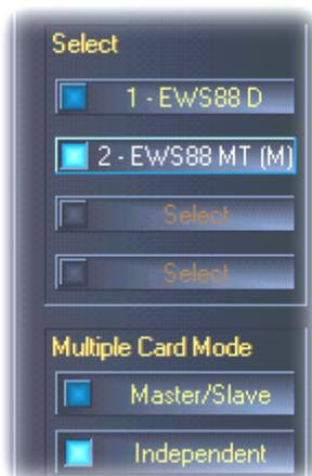
If you select Master/Slave mode, all slave cards are automatically set to external synchronization, as the cards are now digitally synchronized among one another. The clock of the first (master) card is now set to “Internal” (you can choose the cards at the right-hand side of the ControlPanel in the “Select” field).
