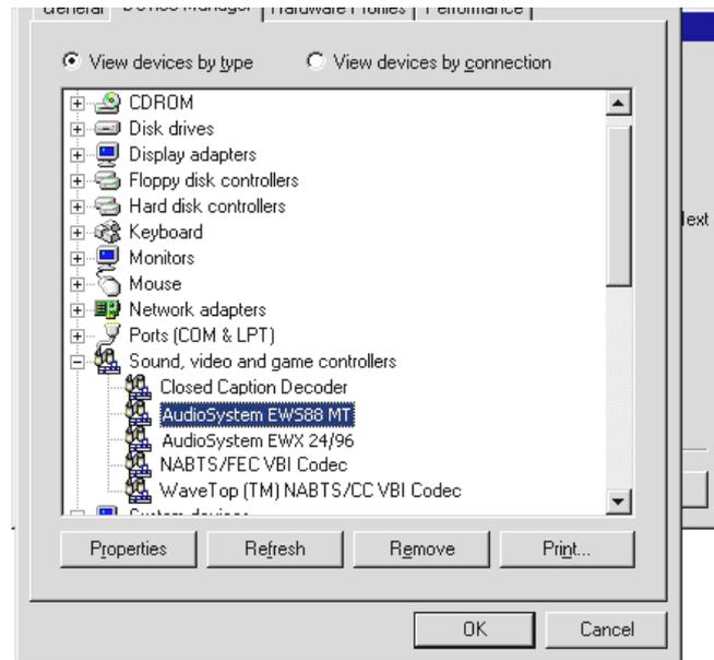
*If everything is correctly set up, the window should look like this. The figure shows the expanded view of the “Sound, video and game controllers” branch. To obtain this view, simply click the “+” symbol on the left side.*
