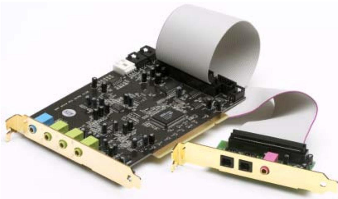
*SoundSystem DMX 6fire LT—PCI card with MRX module*
