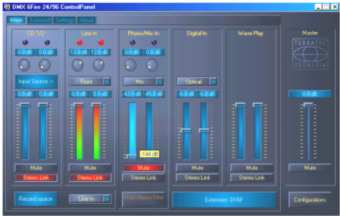
*On the mixer side you can adjust sensitivities and levels, toggle the phono filtering<sup>\*</sup> and select a recording source. The right-hand side of the DMX ControlPanel always remains the same and controls the overall level of the system.*
