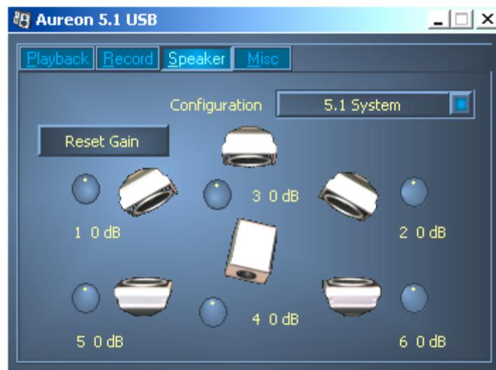
Under each speaker is a label. The first digit (1-6) indicates the output jack of the Aureon 5.1 USB MK II to which that speaker should be connected. The other part of the display (+/- 20 dB) is a readout of the volume dials which are next to each speaker.
