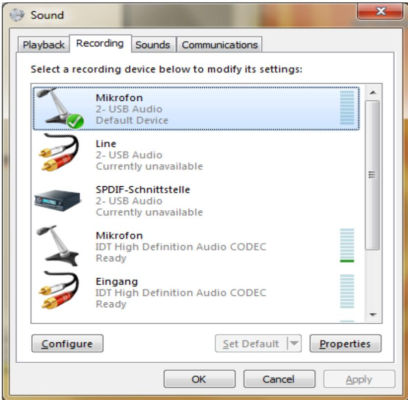
Here you have to set the USB Audio as default device for recording. If you want to use the Line Input as recording device, you have to mark the „Line“-input as default recording device.
