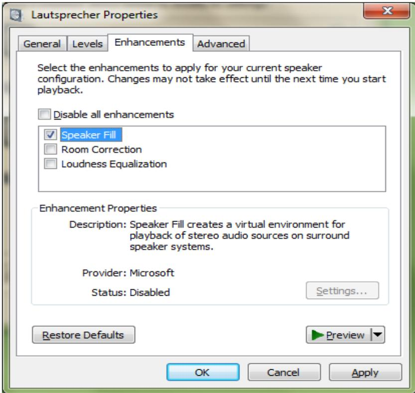
In order to get a stereo signal through all connected speakers, „Speaker Fill“ has to be activated. Click on „Apply“ to finish. In order to use the Aureon 5.1 USB MKII as your default record device, you have to follow the next steps shown below.
