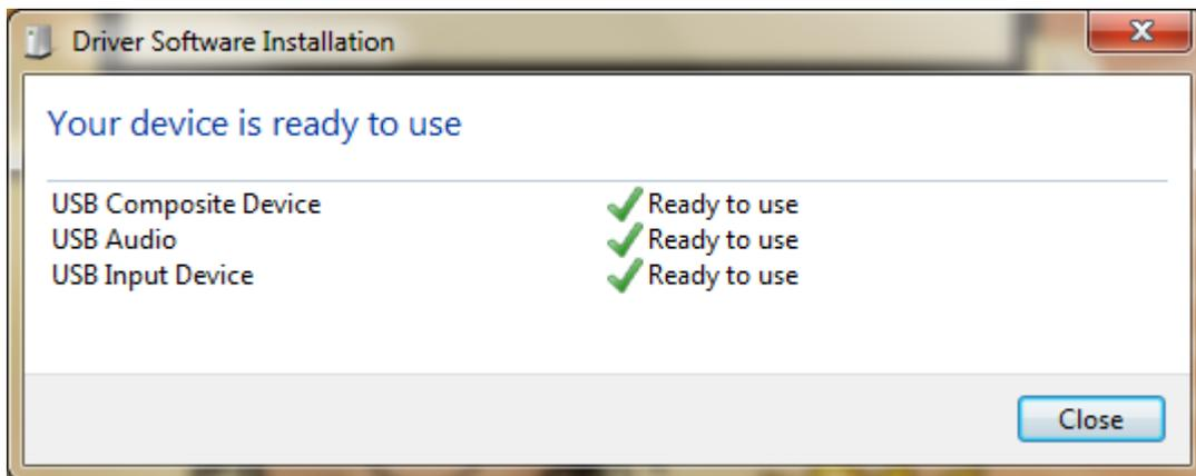
When the installation is done, please check in the Device-Manager if Windows 7 recognized the Soundcard and installed it under Sound, Video and Game Controllers as USB Audio device.
