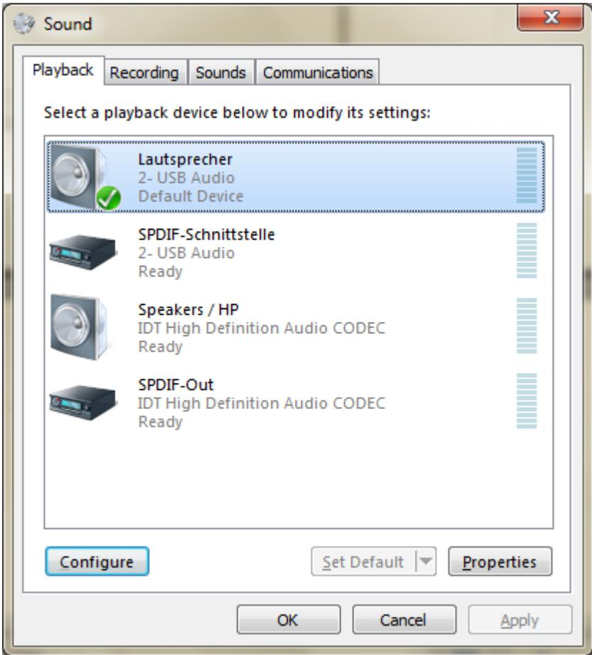
The USB Audio device has to be set as „default Device“. If this is done, click on „Configure“ to enable the 5.1 surround functionality.
