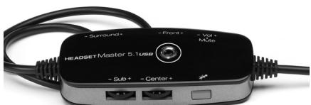
Boot your PC and wait until Windows has loaded completely. Plug the Headset Master 5.1 USB into a free USB port. The blue LED on the controller will light up.
