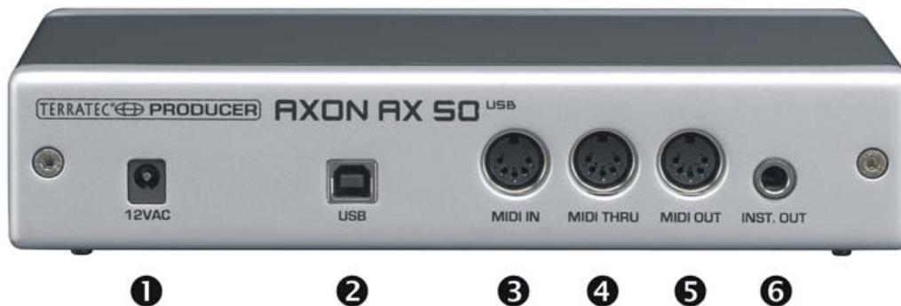
1. 12VAC: Connect the power adapter here (12VAC/1.5A).
